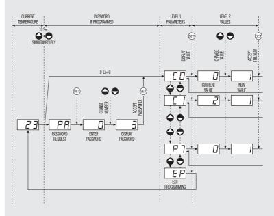
**REMARK:** If no key is pressed for 25 seconds in either of the previous steps, the controller will automatically return to the current temperature display status without modifying any of the parameters values
