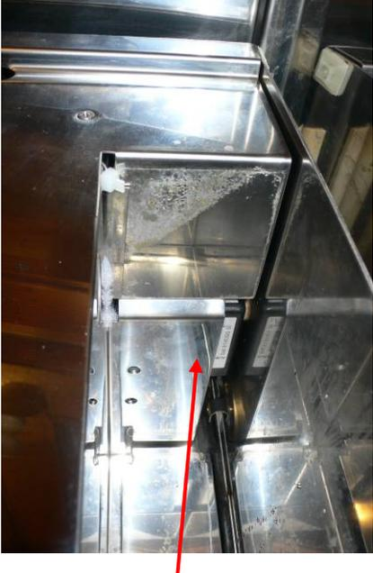
Once the case is on, you can see it is reasonably well protected from water damage. You will need to be more careful when filling the tank
