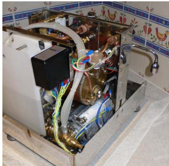
A logical assumption is; the increased heat from the position in the Alex **may** stress the controller more, thus any batch with a weakness may be more likely to become faulty in the Alex, than in a machine where it was located in a cooler position.
