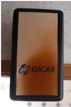
The brown “scorch” mark is actually located above a small 12V transformer that supplies power to the Sirai autofill solenoid (this controls whether water enters the brew circuit or the boiler, a 2 way valve). In both cases the brown mark was in the same place.
