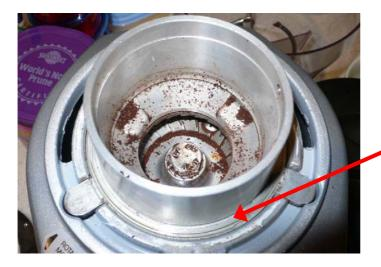
This surface should be lubricated, the adjustment collar bears down on this, give a quick wipe before lubricating
