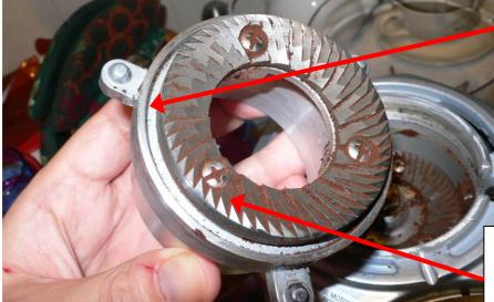
Coffee can collect in this little groove. I have found that if coffee does collect here it can compact. This can make the grinder difficult to move to the fine position, give a false burr touching point and a whining sound. Use a wooden cocktail stick to run around the groove and loosen any coffee
