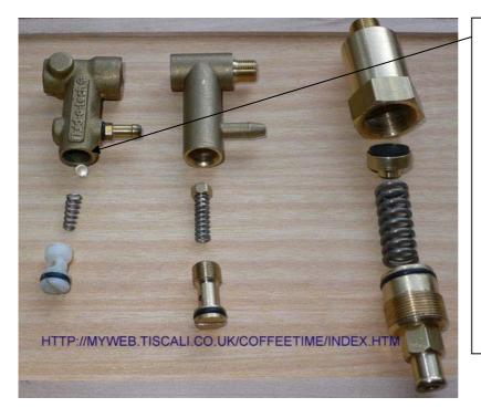
The plastic ball doesn't really inspire confidence as a sealing device. It's actually pressed against a rubber seating held by a brass bush. I didn't bother pulling it out.
