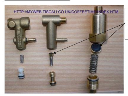
Here we can clearly see the rubber pads on the ends of the brass plungers. The OPV far left uses a plastic ball, which can be seen in the next picture
